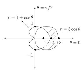
The first step is to determine the intersections of the cardioid  $r = 1 + \cos \theta$  and the circle  $r = 3\cos\theta$ , since this information is needed for the limits of integration. To find points of intersection, we can equate the two expressions for r.
