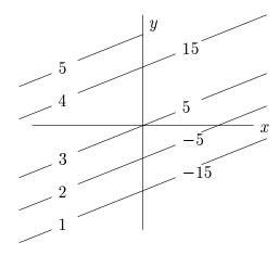
function has a jump along y-axis; the level curves break
